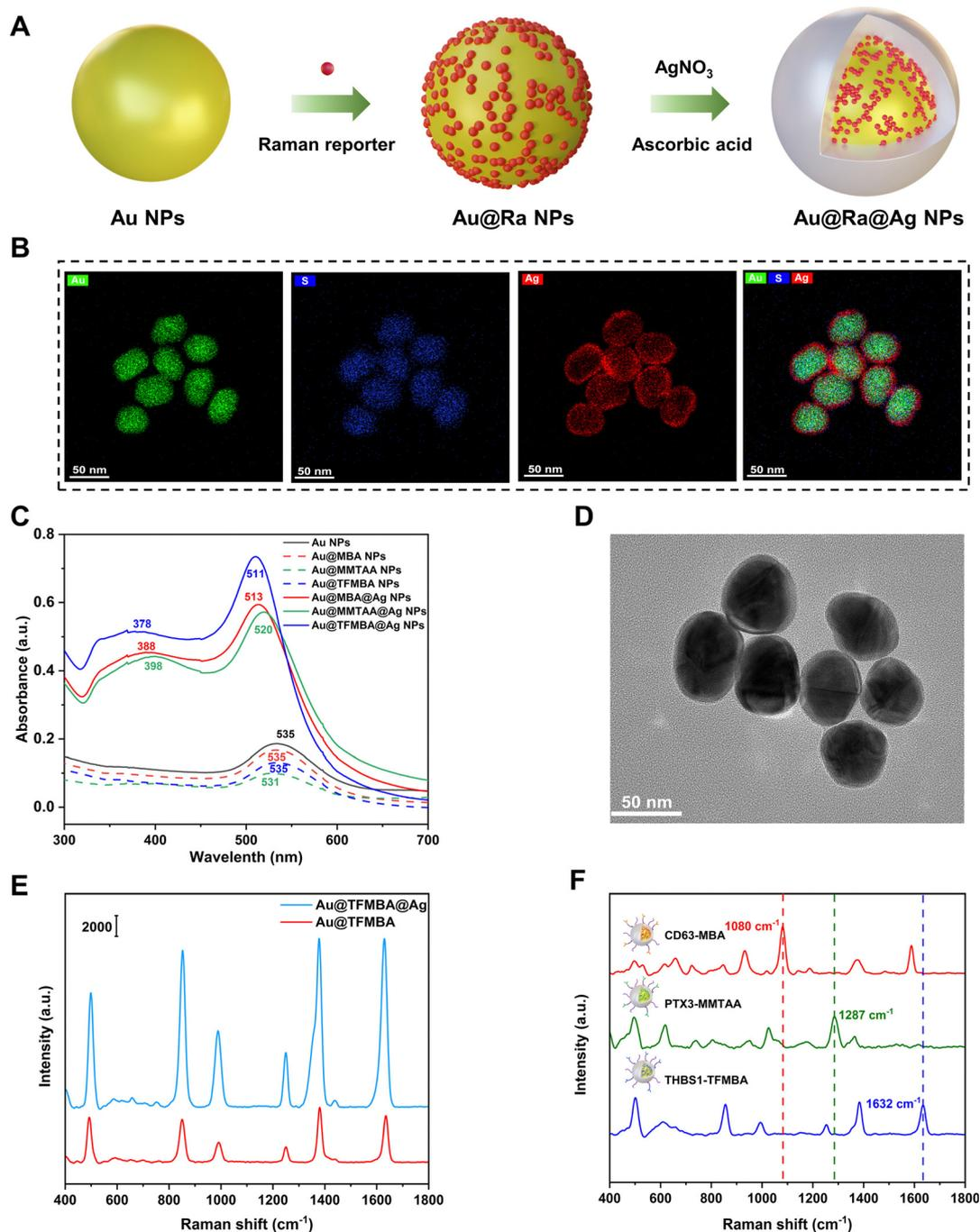
**Fig. 1** Preparation and characterization of SERS nanotags. (A) The synthesis of Au@Ra@Ag NPs using Raman reporter molecules as anchors. (B) EDS mapping of Au@TFMBA@Ag NPs. (C) UV-vis absorption spectra of Au NPs, Au@Ras NPs, and Au@Ras@Ag NPs. (D) A TEM image of Au@TFMBA@Ag NPs. (E) SERS spectra of Au@TFMBA NPs and Au@TFMBA@Ag NPs in water. (F) SERS signals of Au@Ra@Ag NPs with antibody-Raman reporter pairs of CD63-MBA, PTX3-MMTAA, and THBS1-TFMBA.
