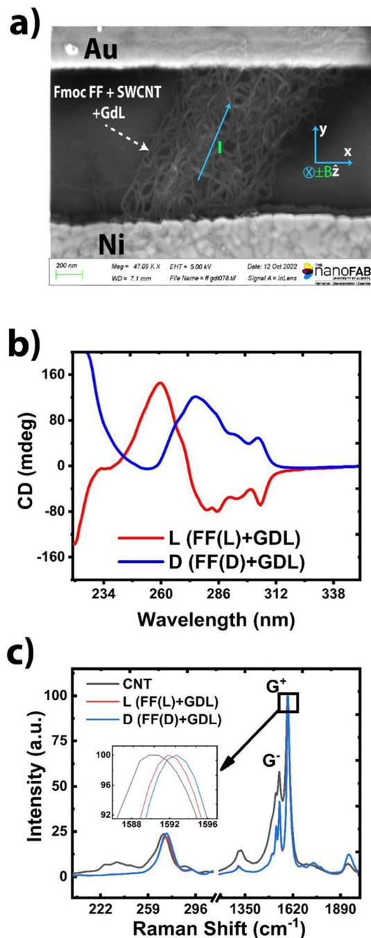
**Fig. 1** (a) SEM image of the two-terminal device. Magnetic field  $B$  is perpendicular to the plane, and hence perpendicular to all the in-plane ( $x$ - $y$ ) current paths. (b) CD spectrum of Fmoc-FF (L/D) hydrogels formed in the presence of GdL. (c) Raman spectrum (532 nm laser), showing the characteristic peaks of CNTs before and after functionalization. The inset shows the shift of the  $G^+$  peak due to functionalization.
