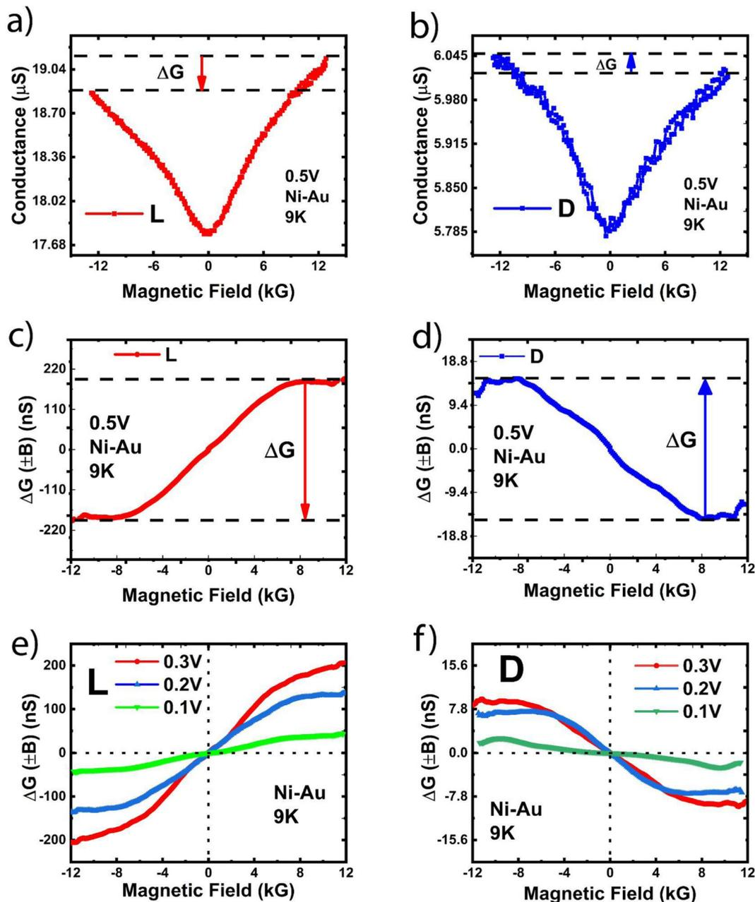
Fig. 4 (a and b) MC measurements on L and D chiral samples, respectively, in the non-linear range ( $\sim 0.5$  V bias). Both forward and backward field scans are recorded. Chirality dependent MC asymmetry is observed, superimposed on a symmetric background positive MC signal. (c and d) Elimination of the background MC signal and  $\Delta G$  vs.  $B$  plots. (e and f)  $\Delta G$  vs.  $B$  as a function of bias, showing that  $\Delta G$  gradually decreases with lowering bias.
