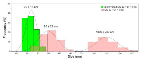
DLS measurements of DC 50 in cell culture medium (DMEM) before and after biotinylation.
