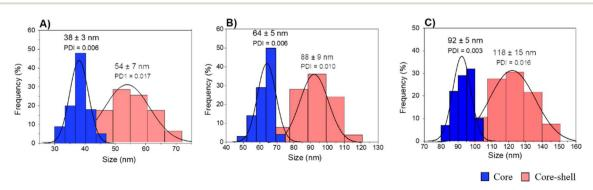
Fig. 3 DLS measurements of core and core-shell silica-based nanosystems in water (A) DC 50, (B) DC 90 and (C) DC 120.
