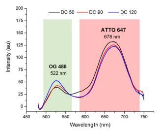
Fig. 4 Normalized fluorescence spectra of DC 50, DC 90 and DC 120 in ethanolic solution ( $\lambda_{ex} = 450$  nm).
