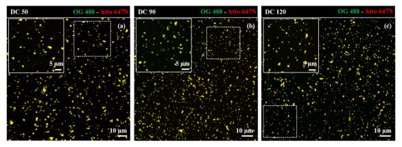
Fig. 6 Confocal imaging of dual-color  $SiO_2$  NPs (a) DC 50, (b) DC 90 and (c) DC 120 immobilized on coverslip. Insets display close-up views (zoom-in) of the regions marked by the dotted white square.
