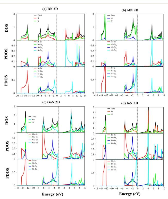
Fig. 7 (a-d) Van Hove singularities of the density of states (DOS) and project-density of states (PDOS) of the BN, AIN, GaN, and InN monolayers, respectively, and those coming from B-/Al-/Ga-/In-/N- orbitals (red, blue, cyan, yellow, and green curves), as well as B-(2s, 2px, 2py, and 2pz), Al- $(3s, 3p_x, 3p_y, and 3p_z)$ ,  $Ga-(4s, 4p_x, 4p_y, and 4p_z)$ ,  $In-(5s, 5p_x, 5p_y, and 5p_z)$ , and  $N-(2s, 2p_x, 2p_y, and 2p_z)$  orbitals (red, green, blue and cyan curves).
