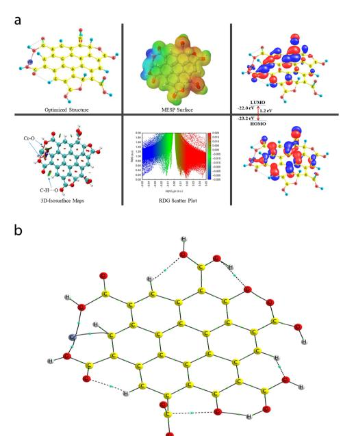
Fig. 8 (a) Optimized structure, MESP surface, HOMO-LUMO 3D maps, 3D-isosurface maps, and RDG scatter plot of Cr<sup>6+</sup> interacting with the functionalized CNP to form the Cr<sup>6+</sup>@CNPt complex at the terminal of the CNP moiety. (b) QTAIM molecular graph of the Cr<sup>6+</sup> ion interacting with the functionalized CNP to form the Cr6+@CNPt complex at the terminal of the CNP moiety.
