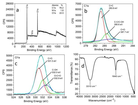
Fig. 2 Full scan XPS spectra (a), high-resolution XPS spectra (b) C 1s region and (c) O 1s region and FTIR spectra (d) of CNPs obtained by the hydrothermal treatment of *Madhuca longifolia* flower.
