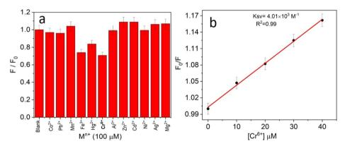
Fig. 5 (a) Fluorescence intensity ratio plot for CNPs in the presence of other heavy metal ions with p-value < 0.05. (b) Calibration plot, CNPs (2.0 mg mL $^{-1}$ ) against Cr $^{6+}$  (0–10  $\mu$ M) ion concentration for the estimation of LOD in the aqueous solution [standard deviation =  $\pm$ 0.043, [M $^{n+}$ ] = 100  $\mu$ M, [CNPs] = 2.0 mg mL $^{-1}$ ,  $\lambda_{exc}$  = 370 nm and  $\lambda_{emi}$  = 454 nm].
