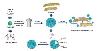
Fig. 1 Formation of the  $Fe_3O_4@SiO_2@NiO$  (FSN)/graphene/ $C_3N_4$  composites.
