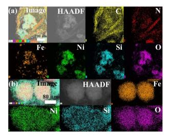
Fig. 3 STEM-HAADF and elemental mapping images of (a)  $Fe_3O_4$ @-SiO<sub>2</sub>@NiO (FSN)/Gr/C<sub>3</sub>N<sub>4</sub> and (b) FSN magnetic nanoparticles (MNPs)—elemental Fe (brown), Ni (green), Si (cyan), O (pink), C (yellow), and N (red) mapping.
