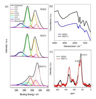
Fig. 1 Characterization of the prepared GO samples. (a) C 1s XPS spectra of GO (3) (GO at pH=3), GO (7) (GO at pH=7) and GO (11) (GO at pH = 11), (b) FTIR spectra GO (3) and GO (11), and (c)  $^{13}$ C NMR spectra of GO (3) and GO (11).
