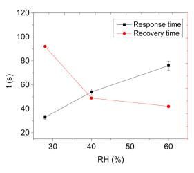
Fig. 9 The response and recovery times versus relative humidity.
