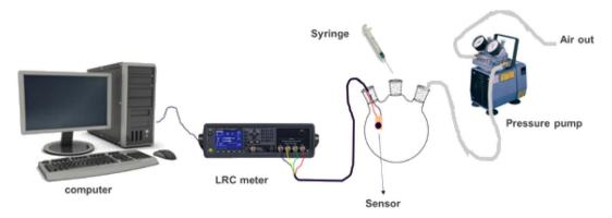
Fig. 1 Gas sensing setup.
