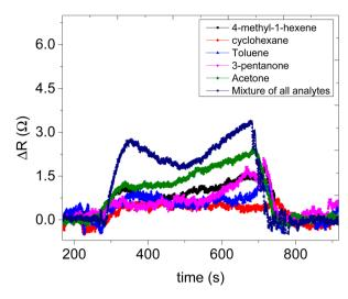
Fig. 11 Static response-recovery curve of sensor 3.
