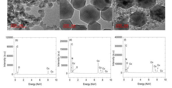
Fig. 3 TEM images of (a) CNPs, (c) ZIF-67 (e) CNPs/ZIF-67 and their respective EDS spectra, (b), (d) and (f).
