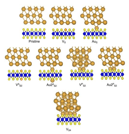
Fig. 2 Optimized geometries with DFT of selected Au/MoS<sub>2</sub> interfaces considered in this work. The pictures were taken in the vicinity of the contact area between the two materials. Interfaces  $V_{S2}^P$  and  $V_{S4}$  refer to MoS<sub>2</sub> with clusters of two and four S vacancies, although following geometry optimization such clusters were fully filled by Au atoms migrating from the above electrode.
