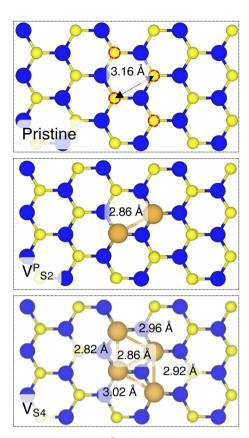
Fig. 5 Top view of pristine,  $V_{S2}^{P}$ , and  $V_{S4}$  interfaces, where the Au electrode was removed for clarity.
