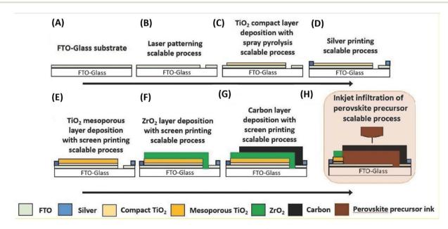
Fig. 11 Pictorial representation of the fabrication of a complete carbon-based PSC. (A–H) Different stages of the fabrication in a scalable process [reproduced from ref. 305 with permission from John Wiley & Sons, Copyright 2016].
