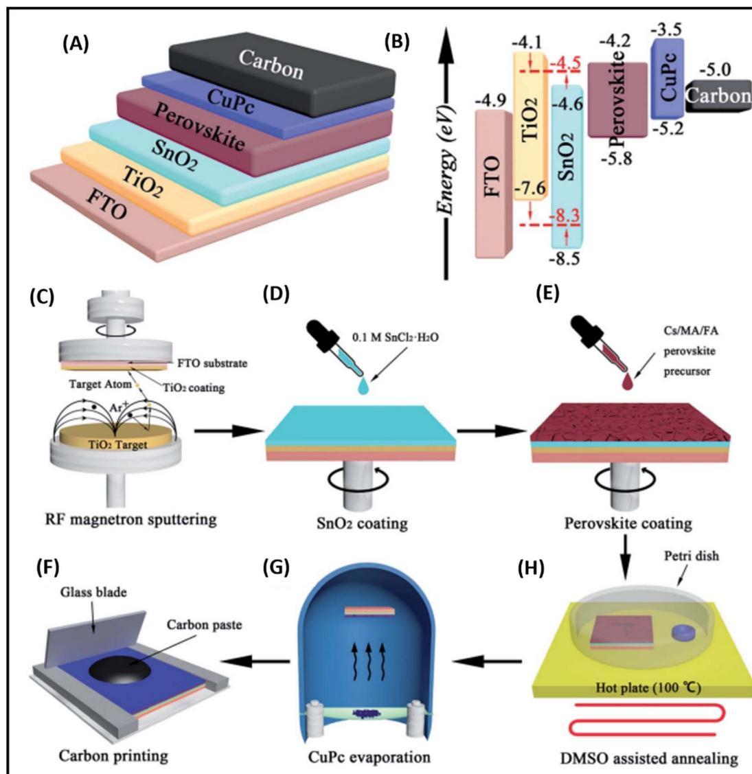
Fig. 9 (A) Device structure of the TiO<sub>2</sub>/SnO<sub>2</sub> ETL-based carbon-PSC, (B) energy level diagram corresponding to the device structure, and (C–H) fabrication process for the commissioning of PSCs [reproduced from ref. 283 with permission from The Royal Society of Chemistry, Copyright 2018].
