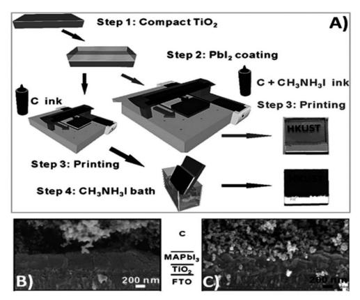
Fig. 5 (A) Process for the fabrication of carbon and CH<sub>3</sub>NH<sub>3</sub>I ink-based PSCs by inkjet printing technique, (B) SEM cross sectional image of carbon ink-based  $TiO_2/CH_3NH_3PbI_3/c$ arbon solar cells, and (C) SEM cross-sectional image of carbon and  $CH_3NH_3I$  ink-based  $TiO_2/CH_3NH_3PbI_3/c$ carbon solar cells [reproduced from ref. 193 with permission from John Willey & Sons, Copyright 2014].
