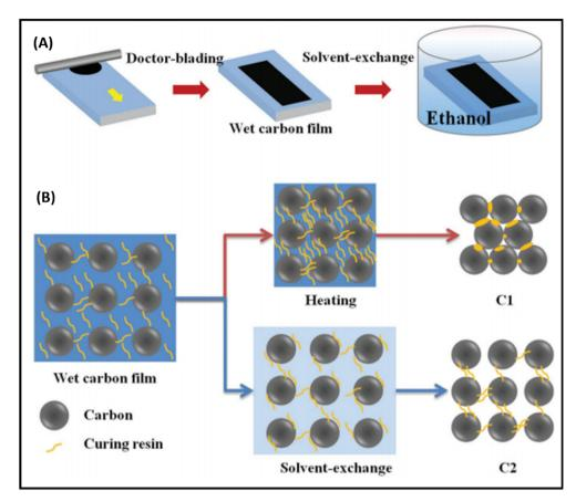
Fig. 6 (A) Solvent-exchange method for the preparation of C2 films. (B) Mechanism of microscopic curing for the formation of C1 and C2 films [reproduced from ref. 194 with permission from John Willey & Sons, Copyright 2018].
