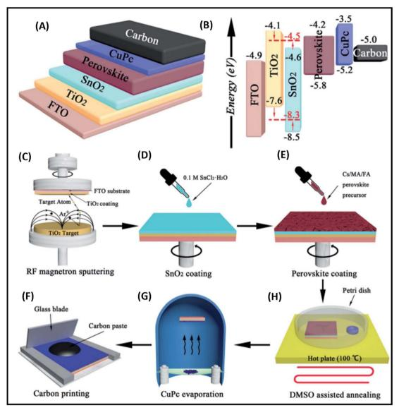
$\textbf{Fig. 9} \hspace{0.3cm} \textbf{(A) Device structure of the TiO}_2/SnO}_2 \hspace{0.1cm} \textbf{ETL-based carbon-PSC, (B) energy level diagram corresponding to the device structure, and (C-H)}_2 \hspace{0.1cm} \textbf{(C-H)}_2 \hspace{0.1cm} \textbf{(C-H)}_3 \hspace{0.1cm} \textbf{$ fabrication process for the commissioning of PSCs [reproduced from ref. 283 with permission from The Royal Society of Chemistry, Copyright 2018].
