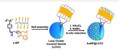
Scheme 1 Preparation process of the composite vesicle (AuNP@LCCV) containing AuNPs with a particle size of less 3 nm by self-assembly of comb-like block copolymer c-iEP (l=104, m=50, n=48) and in situ reduction of Au ions in the loop corona of the LCCV vesicle.
