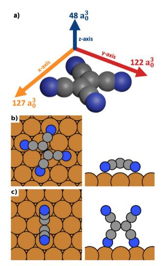
Fig. 1 (a) TCNE and its polarizabilities in different directions (given by the length of the arrows and the number next to the arrows). (b) The most stable lying adsorption geometry (in absence of an electric field). (c) The most stable standing adsorption geometry (in absence of an electric field).
