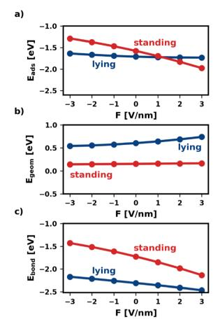
Fig. 2 Adsorption energy of isolated molecules and their components as function of the electric field. Only the most stable adsorption geometry for every category is shown. (a) shows the total adsorption energy, (b) shows the component that corresponds to geometric changes during adsorption (reorientation, deformation, etc.), and (c) shows the component that stems from the bonding of the deformed and reoriented molecule with the substrate
