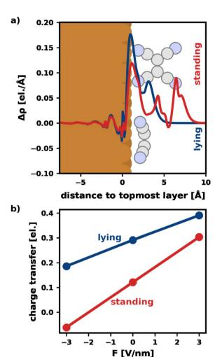
Fig. 3 Visualization of the charge transfer. (a) Plane-averaged electron density difference between a field  $F=3~\rm V~nm^{-1}$  and  $0~\rm V~nm^{-1}$  for the most stable lying/standing adsorption geometries. The spatial extent of adsorption geometries of a lying and a standing molecule are indicated. (b) Net charge transfer into the molecule (calculated *via* Mulliken analysis) for the most stable lying/standing adsorption geometry.
