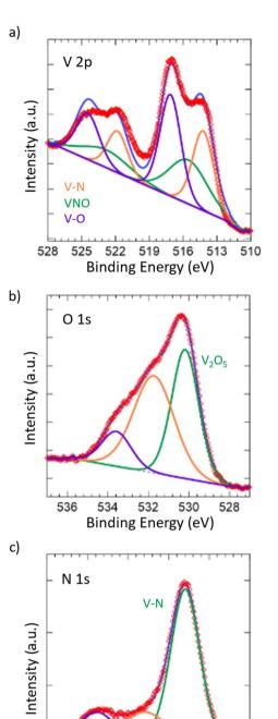
Fig. 2 XPS spectra of (a) V 2p, (b) O 1s, and (c) N 1s for the synthesized VN. All spectra were plotted with respect to reference values. The degree of surface oxidation and amount of pristine vanadium nitride structure were tracked according to the V 2p, O 1s, and N 1s spectra.
