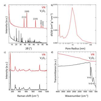
Fig. 1 Physical characterization of high surface area passivated VN powder using (a) XRD for bulk characterization, (b) N<sub>2</sub>-physisorption for pore size distribution, and (c) Raman and (d) FTIR spectroscopies for surface characterization.
