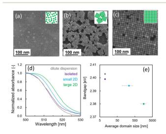
Fig. 2 (a-c) SEM images with schematic illustrations, (d) UV absorption edges, and (e)  $E_g$  as a function of the domain size in NC arrays; (a) isolated NCs, (b) small 2D arrays, and (c) large 2D arrays.
