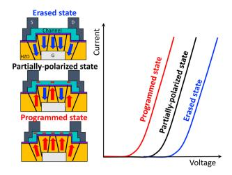
Fig. 1 Schematic operation principles of the  $V_{\rm th}$  compensation using a FeTFT.
