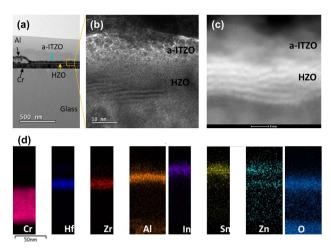
Fig. 4 (a) TEM image of S/D and channel regions. (b) TEM, (c) STEM, and (d) EDS images of an a-ITGO/Al $_2O_3$ /HZO/Cr FeFET.
