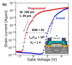
Fig. 7 (a) Polarization-voltage (P-V) hysteresis and current-voltage (I-V) curves of the Cr/HZO/Al<sub>2</sub>O<sub>3</sub>/Al MFIM capacitor and (b)  $I_D-V_G$ characteristics of the a-ITZO FeTFT.
