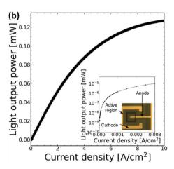
Fig. 9 (a) Current density–voltage characteristics and (b) light output power–current density characteristics of AlGaInP/GaInP MQW LEDs with various device sizes.
