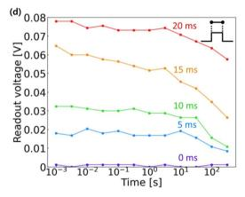
Fig. 8 (a) Block diagram of the measurement setup. (b) Schematic diagram when the channel is not formed or formed. (c) Input and readout voltage vs. time. (d) Retention properties with various pulse times.
