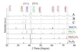
Fig. 4 XRD patterns of  $Mn_xFe_{3-x}O_4$  NFs prepared from [Mn(acac)<sub>3</sub>]/[Fe(acac)<sub>3</sub>] ratio equal to (A) 1 and (B) 3 at 200 °C, (C) 7 at 250 °C. A secondary phase matched MnCO<sub>3</sub> (Reference ICDD PDF card no. 00-044-1472) was found for NFs prepared from a precursor ratio equal to 7 at 250 °C. No detected peaks matched  $Mn_3O_4$  (PDF card no. 01-080-0382).
