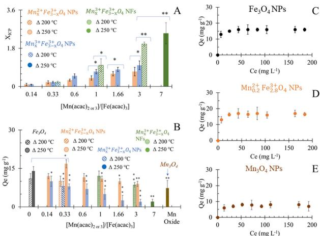
Fig. 5 (A) Elemental analysis of  $Mn_xFe_{3-x}O_4$  NS that were prepared at 200 °C and 250 °C. \*P < 0.05 and \*\*P < 0.01 in comparison to  $Mn_x^{3+}Fe_{3-x}^{3+}O_4$  NPs of similar precursor ratios; (B) adsorption capacity of NPs for  $Cr^{6+}$ , \*P < 0.05 and \*\*P < 0.01 in comparison to  $Fe_3O_4$  NPs; (C)–(E) adsorption isotherm of  $Cr^{6+}$  by  $Fe_3O_4$ ,  $Mn_{0.2}^{2+}Fe_{2.8}^{3+}O_4$  and  $Mn_3O_4$  NPs respectively.
