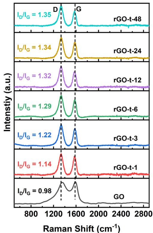
Fig. 5 Raman spectra of GO and rGO prepared with various reduction times.
