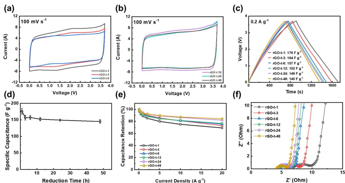
Fig. 8 CV curves at voltage sweep rate of 100 mV s<sup>-1</sup> of graphene synthesized with reduction time of (a) 1 h, 3 h, and 6 h; (b) 12 h, 24 h, and 48 h; (c) charge–discharge curves, (d) specific capacitance, (e) rate performance, and (f) Nyquist plots of supercapacitors with rGOs synthesized with different reduction times.
