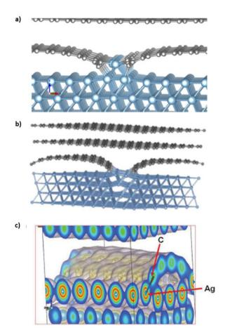
Fig. 8 Optimized structure of (a) a solid graphene-aluminum covetic<sup>20</sup> (b) and solid graphene-silver covetic.<sup>21</sup> (c) Electron density spectrum showing the bonding between graphene and silver at the graphene edge,<sup>21</sup> (a) has been reproduced from ref. 20 with permission from Elsevier, copyright 2016, (b) and (c) have been reproduced from ref. 21 with permission from Wiley, copyright 2015.
