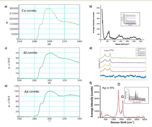
Fig. 7 EELS and Raman spectra of (a and b) copper,<sup>20,40</sup> (c and d) aluminum,<sup>3,20</sup> and (e and f) silver covetics,<sup>20,40</sup> (a, d), and (f) have been reproduced from ref. 20 with permission from Elsevier, copyright 2016, (c) has been reproduced from ref. 3 with permission from TechConnect, copyright 2012.
