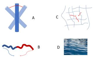
**Fig. 3** Different types of relaxation processes. (A) Rotational diffusion of rod-like particles along minor semi-axes; (B) internal motion of long flexible macromolecules; (C) gel mesh size fluctuations; (D) hydrodynamic modes in a plain solvent.
