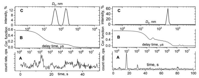
Fig. 2 Example of poor-quality measurements: typical count rate (A), correlation function (B), and D<sub>h</sub> distribution function (C) for samples containing dust or large aggregates (left); and for even the worst case of system sedimentation (right).
