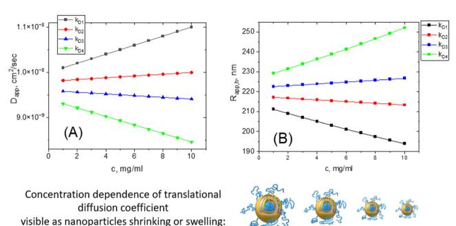
Fig. 7 The example of concentration dependence of apparent translational diffusion coefficient for different k<sub>D</sub> values (A); the concentration dependence of apparent hydrodynamic radii calculated from  $D_{t}$  (B).
