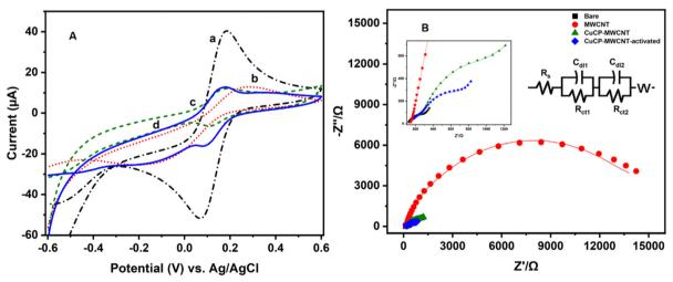
Fig. 3 (A) CV of the bare SCPE (curve a) after MWCNTs functionalization (curve b) showed a decrease in the redox response, and then the electrodeposited CuCP-modified electrode (curve c) after electrochemical stabilization (curve b) showed an increase in the redox response of the CuCP-modified MWCNTs-SPCE and its corresponding EIS (B) in the 5 mM  $K_3[Fe(CN)_6]$  containing 0.1 M KCl solution.
