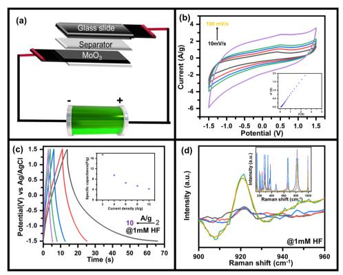
Fig. 4 (a) Schematic diagram of as-fabricated MoO<sub>3</sub>//AC supercapacitor device, (b) CV curves measured at scan rates of 10 to 100 mV s<sup>-1</sup> along with the corresponding EIS plot (ESI†), (c) GCD plots at 2 A g<sup>-1</sup> to 10 A g<sup>-1</sup> along with variation of specific capacitance as a function of current density (inset) and (d) *in situ* Raman spectra of asymmetric supercapacitor device during the charging and discharging process.
