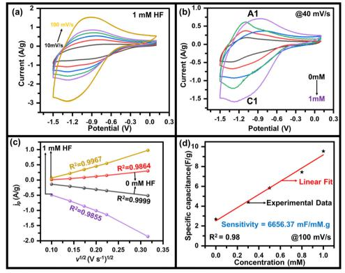
Fig. 2 CV graph of  $MoO_3$  at GCE with (a) 1 mM HF, (b) 0 mM, 0.2 mM, 0.5 mM, 0.8 mM, and 1.0 mM HF in 0.5 M LiClO<sub>4</sub> in PC, (c) variation of current density ( $j_0$ ) vs.  $v^{1/2}$  graph with and without HF, and (d) variation of specific capacitance with concentration of HF including raw data and linear fit.
