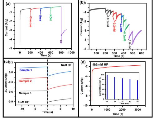
Fig. 3 Chronoamperometric response of MoO<sub>x</sub>/CC (a) upon the addition of 1 mM HF, glucose, urea, and KOH, (b) upon the addition of different concentrations of HF (0.1, 02, 0.3, 0.5, and 1.0 mM). (c) Response time of the sensor for three different batches of the sample under 1 mM HF, and (d) long-term stability (inset: current retention versus time graph) test of the MoO<sub>3</sub>/CC electrode.
