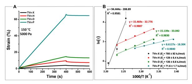
Fig. 6 (A) Creep-recovery experiments for networks crosslinked with m-xylylenediamine (TVn-X), hexamethylenediamine (TVn-H), diaminododecane (TVn-D), and Priamine (TVn-P) at 150 °C at a constant force of 5000 Pa (experiments ran in duplicate). (B) Arrhenius plots of stress relaxation data for networks ( $\tau$  at  $G/G_0 = 1/e$ , in 5 °C increments). Data indicates flow behavior is dependent on diamine functionality. Vitrimer samples in triplicate.
