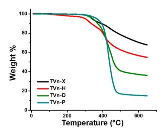
Fig. 4 Thermogravimetric analysis (TGA) plots (under N<sub>2</sub>) of networks crosslinked with m-xylylenediamine (TVn-X), hexamethylenediamine (TVn-H), diaminododecane (TVn-D), and Priamine (TVn-P) indicating excellent stability and outstanding charring behavior.
