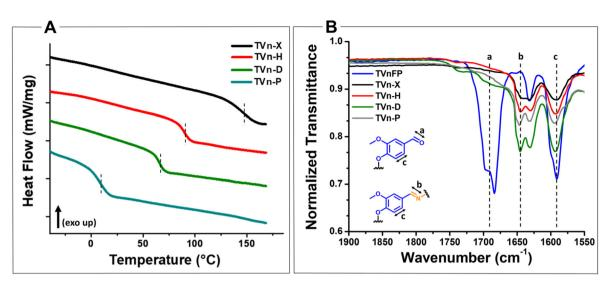
Fig. 3 (A) Stacked differential scanning calorimetry (DSC) plots with marked  $T_g$  values of networks crosslinked with m-xylylenediamine (TVn-X), hexamethylenediamine (TVn-H), diaminododecane (TVn-D), and Priamine (TVn-P) showing excellent tunability over a wide temperature range. (B) Overlayed FTIR spectra of vitrimers with trivanillin monomer (TVnFP), indicating near full disappearance of the aldehyde carbonyl stretch and clear emergence of characteristic imine stretch.
