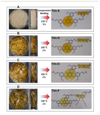
Fig. 2 Compression molding of vitrimer particles from networks of trivanillin monomer crosslinked with (A) *m*-xylylenediamine (TVn-X), (B) hexamethylenediamine (TVn-H), (C) diaminododecane (TVn-D), and (D) Priamine (TVn-P). Resultant disk and bar geometries indicate excellent healability with minimal defects and high transparency.
