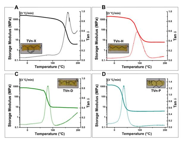
Fig. 5 DMA thermograms of networks crosslinked with (A) m-xylylenediamine (TVn-X), (B) hexamethylenediamine (TVn-H), (C) diaminododecane (TVn-D), and (D) Priamine (TVn-P) showing  $tan(\delta)$  peaks consistent with  $T_q$  values from DSC and constant rubbery plateau moduli indicating constant crosslink density. Inset images of vitrimer bar used in experiments.
