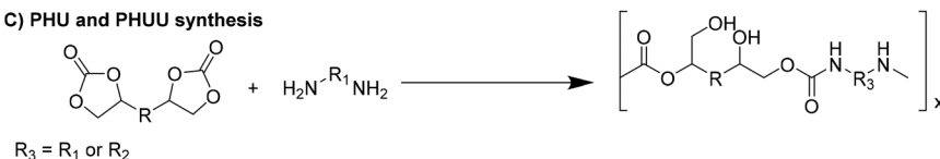
Fig. 11 Polyhydroxyurethane (PHU) and PHUU synthetic route.
