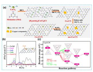
Fig. 23 (a) Schematic diagram of the synthesis process over Cu-CCN samples by using the melamine and CuCl2 as a pre structure of the as-prepared samples. (b) The model of the introduction of a single Cu atom into carbon nitride. (c) Reaction pathways for photocatalytic CO2 reduction and the corresponding chemical molecular structure on Cu-CCN samples based on DFT calculation. 92
