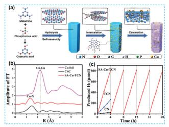
Fig. 21 (a) Schematic illustration of the preparation of SA-Cu-TCN. (b) Fourier transform (FT) of the  $k^2$ -weighted Cu K-edge EXAFS (phase shift not corrected) of SA-Cu-TCN, CSC, CuO, and Cu foil. (c) Temporal H<sub>2</sub> evolution under visible light irradiation ( $\lambda > 420$  nm).<sup>89</sup>
