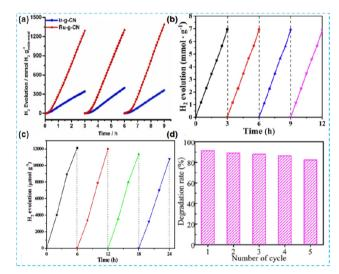
**Fig. 31** (a) Photocatalytic test cycles of Ir-g-CN and Ru-g-CN under light irradiation.  $^{64}$  (b) Cycling tests of the photocatalytic hydrogen evolution of 1.0%-Pt/CN-BH-H.  $^{127}$  (c) Photocatalytic H<sub>2</sub>-production of 24 h on the NiSCN5 photocatalyst with evacuation every 6 h.  $^{117}$  (d) TC degradation efficiency over five cycles.  $^{135}$
