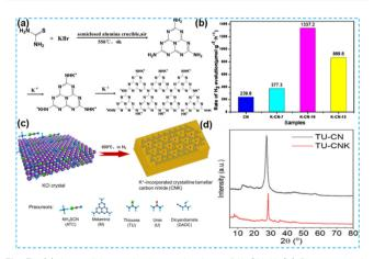
Fig. 3 (a) A possible synthetic mechanism of K-CN-X. (b) Photocatalytic activity of K-doped CN toward the HER from water. 33 (c) Synthesis of CNK frameworks (ATC-CNK, M-CNK, TU-CNK, U-CNK, and DCDA-CNK) on KCl crystals. (d) X-ray diffraction profiles of ATC-CN and ATC-CNK.34
