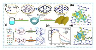
Fig. 28 (a) Illustration of the synthetic process used in producing InCu/PCN. (b) Illustration of the synthetic process used in producing  $InCu/PCN.^{113}$  (c) Schematic diagram of the prepared process for InCNand CulnCN. (d) UV-Vis absorption spectra. (e) Charge density. 114
