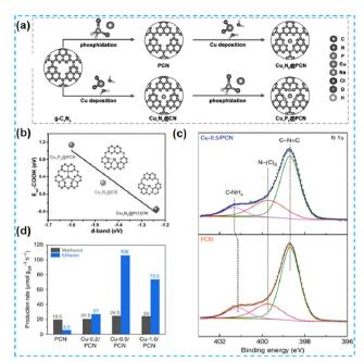
Fig. 20 (a) Scheme of the synthesis of  $Cu_1N_3$ @PCN and  $Cu_1P_3$ @PCN. (b) The relationship between the d band center and adsorption energy of COOH\* on single Cu sites of three model catalysts. <sup>87</sup> (c) N 1s XPS spectra of PCN and Cu-0.5/PCN. (d) Liquid products of methane conversion over PCN and Cu-X/PCN. <sup>88</sup>
