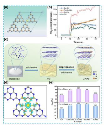
Fig. 10 (a) Schematic model of Pd-Cv-CN: Pd (yellow), N (blue), and C (orange). (b) NO<sub>2</sub> generation.<sup>56</sup> (c) Synthesis and structural characterization of CN, 0.1CNPd and 0.3CNPd. (d) The charge density distribution differences between CN and CNPd. (e)  $\eta$ NO.<sup>57</sup>
