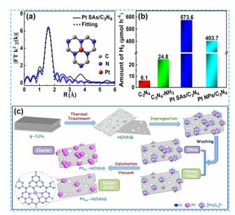
(a) EXAFS fitting Pt curve for Pt SAs/C<sub>3</sub>N<sub>4</sub>. (b) Photocatalytic  $H_2$  evolution activities over  $C_3N_4$ ,  $C_3N_4$ -N $H_3$ , Pt SAs/ $C_3N_4$ , and Pt NPs/  $C_3N_4$ . (c) Schematic of the Pt<sub>Cl</sub>-HCNNS and Pt<sub>SA</sub>-HCNNS fabrication. <sup>45</sup>
