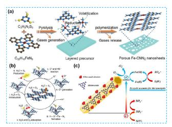
Fig. 32 (a) Fabrication scheme of Fe-CNN $\chi$ . (b) Catalytic reaction mechanism of H<sub>2</sub>S selective oxidation on Fe-CNN $\chi$ . <sup>143</sup> (c) Schematic illustration of mechanisms for S(IV) activation by MF2 under visible light irradiation. <sup>70</sup>
