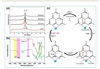
Fig. 4 (a) XRD patterns of K<sup>+</sup>-Na<sup>+</sup> codoped CN.<sup>35</sup> (b) FT-IR of CN and Rb doped CN (CNR-0.5). (c) Proposed mechanism of the two-step single-electron  $O_2$  reduction reaction pathways on CNR-0.5.<sup>36</sup>
