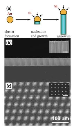
Fig. 4 (a) Schematic diagram of VLS growth of Si nanowires. Reproduced with permission from ref. 60, © 2006 IOP Publishing Ltd Side-view (b) and top-view (c) SEM images of a Au-catalyzed Si wire array. Reproduced with permission from ref. 62, © 2007 American Institute of Physics.
