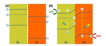
Fig. 21 Schematic diagram of the energy band diagram of a Z-scheme heterojunction, (a) in the dark before contact, (b) under illumination after
