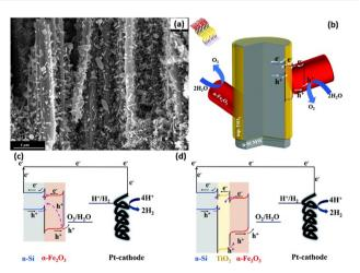
Fig. 24 SEM image (a) and schematic diagram (b) of the n-Si nanowires/  $TiO_2/\alpha$ -Fe<sub>2</sub>O<sub>3</sub>. Band alignment of n-Si/ $\alpha$ -Fe<sub>2</sub>O<sub>3</sub> (c) and n-Si/ $TiO_2/\alpha$ -Fe<sub>2</sub>O<sub>3</sub> (d). Reproduced with permission from ref. 155, Copyright © The Royal Society of Chemistry 2020.
