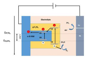
Fig. 18 Schematic diagram of energy band alignment of the Si/g-C<sub>3</sub>N<sub>4</sub> heterojunction. Reproduced with permission from ref. 135, Copyright © 2016 Published by Elsevier B.V.
