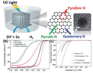
Fig. 17 (a) Schematic of N-doped graphene quantum sheets (N-GQSs) decorated on a Si nanowire photocathode electrode. (b) Photoelectrochemical and (c) electrochemical HER performance of the planar and 1D nanostructured Si photoelectrodes with/without N-GQS catalysts. Reproduced with permission from ref. 131, Copyright © The Royal Society of Chemistry 2015.
