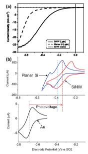
Fig. 9 (a) PEC HER performance comparison of the Si nanowire and planar Si. (b) Cyclic voltammetry curves of methylviologen on the Si nanowire and planar Si photoelectrode under illumination and on the Au electrode in the dark. Reproduced with permission from ref. 81, Copyright © 2012, American Chemical Society
