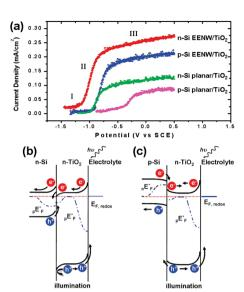
Fig. 22 (a) PEC OER performance on different Si/TiO<sub>2</sub> photoelectrodes. Band structures diagram of the n-Si/n-TiO<sub>2</sub> (b) and p-Si/n-TiO<sub>2</sub> heterostructures. Reproduced with permission from ref. 143, Copyright © 2009, American Chemical Society.
