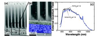
Fig. 13 (a and b) SEM images of the Ni-Mo/TiO<sub>2</sub>/n<sup>+</sup>p-Si microwire array, (c) spectral response data for the best-performing n<sup>+</sup>p-Si microwire-array photocathode loaded with Ni-Mo and TiO2 scattering particles (blue curve) and for the best-performing n+p-Si microwire-array photocathode loaded with Pt and TiO<sub>2</sub> scattering particles (black curve). Reproduced with permission from ref. 93, Copyright © The Royal Society of Chemistry 2015.
