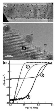
Fig. 10 (a) TEM and (b) HRTEM images of Pt nanoparticles modified Si nanowire, (c) PEC HER performance of naked Si nanowires (11), and Si nanowires modified with Pt nanoparticles prepared by ELD (2) and ALD (3). Reproduced with permission from ref. 86, Copyright © 2013 Wiley-VCH Verlag GmbH & Co. KGaA, Weinheim.
