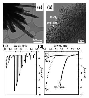
Fig. 15 TEM (a) and HRTEM (b) images of the MoS<sub>2</sub>/Si nanowires. Comparation of the photoelectrochemical HER performance: (c) Si nanowires and MoS<sub>2</sub>/Si nanowires, (d) Si nanowires modified with MoS<sub>2</sub> or Pt nanoparticles in the dark or under illumination. Reproduced with permission from ref. 99, Copyright © 2012 Wiley-VCH Verlag GmbH & Co. KGaA, Weinheim
