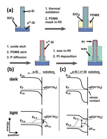
Fig. 26 (a) Schematic diagram of the preparation process of Pt/n+p-Si wire arrays. Band bending of (b) p-Si and (c) n+p-Si photocathodes in contact with electrolyte. Reproduced with permission from ref. 68, Copyright © 2011, American Chemical Society.
