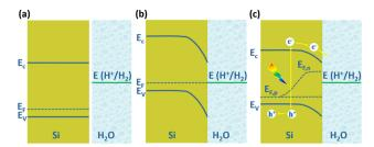
Fig. 1 Schematic diagram of Si/electrolyte interface. (a) Before contact, (b) equilibrium reached after contact in the dark, (c) under illumination.
