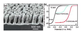
Fig. 16 (a) SEM image of the p-Si/NiCoSe<sub>x</sub> core/shell nanopillar array, (b) PEC HER performance. Reproduced with permission from ref. 120, Copyright © The Royal Society of Chemistry 2016.
