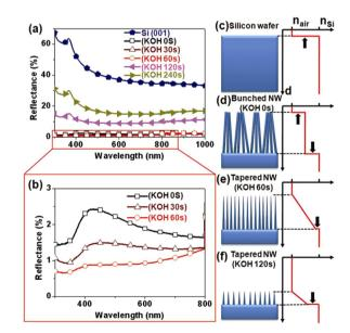
Fig. 7 (a and b) Optical reflective spectra recorded from different samples. (c-f) Schematic representation of the correlation between Si nanowire morphology and effective refractive index profile. Reproduced with permission from ref. 77, Copyright © 2011, The Optical Society.
