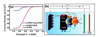
Fig. 20 (a) PEC HER performance of the p-SiNWs-Ta<sub>2</sub>O<sub>5</sub>-NGQD photoelectrodes. (b) Schematic diagram of the charge transfer process in the p-SiNWs-Ta<sub>2</sub>O<sub>5</sub>-NGQD photoelectrode. Reproduced with permission from ref. 141, Copyright © The Royal Society of Chemistry 2022.
