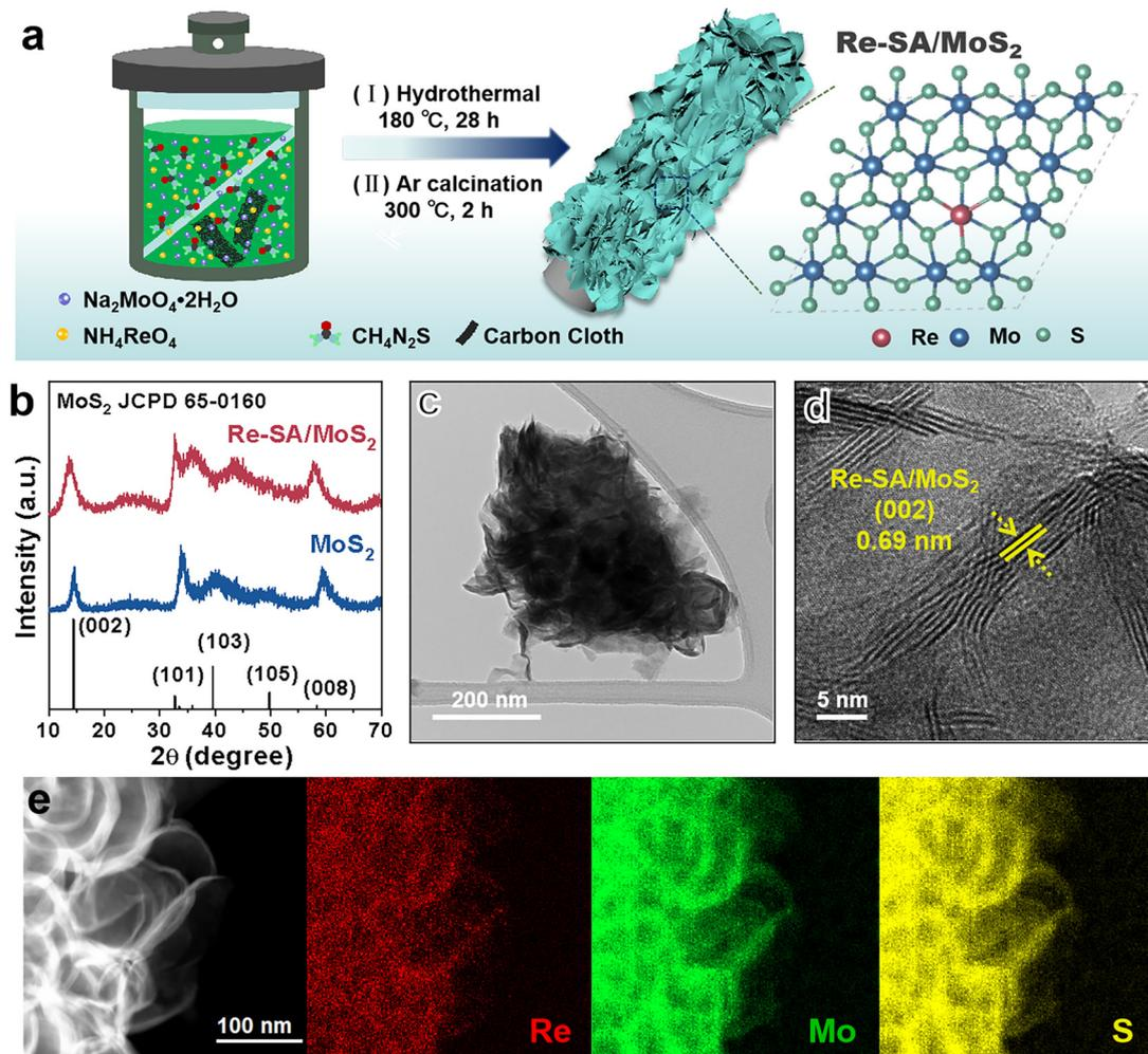
**Fig. 1** (a) Schematic illustration of the fabrication of the Re-SA/MoS<sub>2</sub> catalysts. (b) XRD patterns of the fabricated MoS<sub>2</sub> and Re-SA/MoS<sub>2</sub> catalysts. (c and d) TEM and HRTEM images of the Re-SA/MoS<sub>2</sub> catalyst. (e) EDS mapping of the Re-SA/MoS<sub>2</sub> catalyst.
