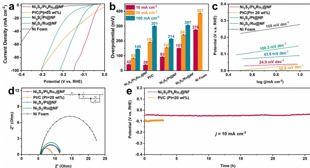
Fig. 3 Electrocatalytic HER performance in 0.1 M HClO<sub>4</sub> solution. (a) Polarization curves of the electrocatalysts for the HER (with 95% iR compensation), (b) the resultant overpotentials at current densities of 10, 50 and 100 mA cm<sup>-2</sup> for the as-prepared electrocatalysts, (c) the corresponding Tafel plots, (d) Nyquist plots under open-circuit voltage, and (e) long-term stability test at current densities of 10 mA cm<sup>-2</sup>.
