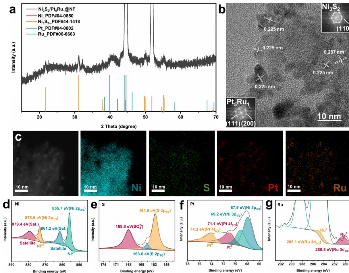
Fig. 1 Structural and microstructure characterizations of  $\text{Ni}_3\text{S}_2/\text{Pt}_5\text{Ru}_1@\text{NF}$ . (a) XRD pattern, (b) HRTEM image and the corresponding FFT patterns, (c) STEM image and the corresponding EDX elemental mapping images, and XPS spectra of (d) Ni 2p, (e) S 2p, (f) Pt 4f, and (g) Ru 3d.
