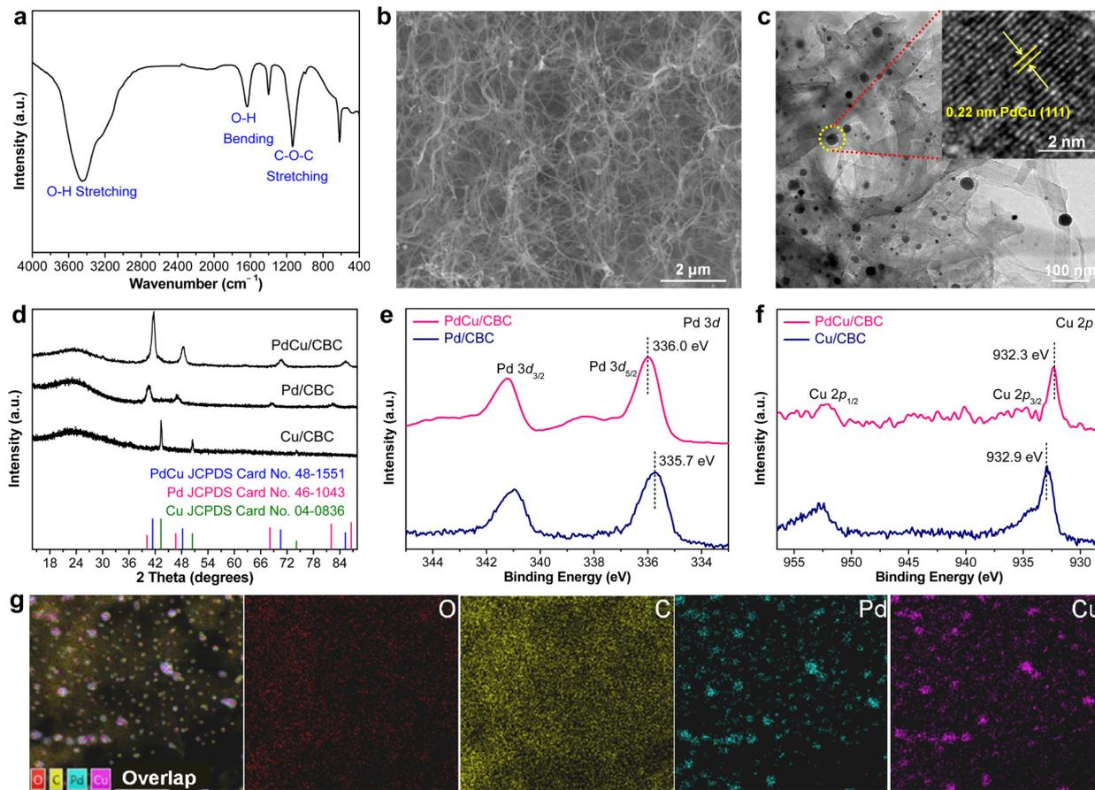
**Fig. 1** (a) FT-IR spectrum of BC. (b) SEM and (c) TEM images of the PdCu/CBC. (d) XRD patterns of the Pd/CBC, Cu/CBC and PdCu/CBC. (e) Pd 3d XPS spectra of the Pd/CBC and PdCu/CBC. (f) Cu 2p XPS spectra of the Cu/CBC and PdCu/CBC. (g) Corresponding elemental mapping images of the PdCu/CBC.
