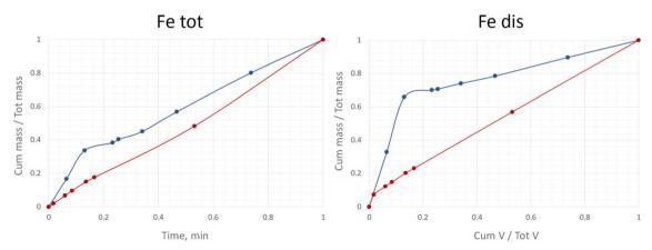
Fig. 6 First flush graphical analysis of the ratio runoff mass fraction and volume fraction for two rainfall events.
