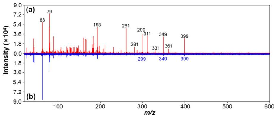
Fig. 6 Matrix-free LDI-MS for direct analysis of (a) a wastewater sample without pretreatment and (b) a filtered sample solution after performing CB adsorption. Note:  $m/z$  281 and 331 were assigned as the characteristic peaks of PFOA.  $m/z$  299, 349 and 399 were assigned as the characteristic peaks of PFOS.
