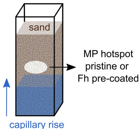
Fig. 1 Schematic setup of a sample container filled with sand and MP hotspot.
