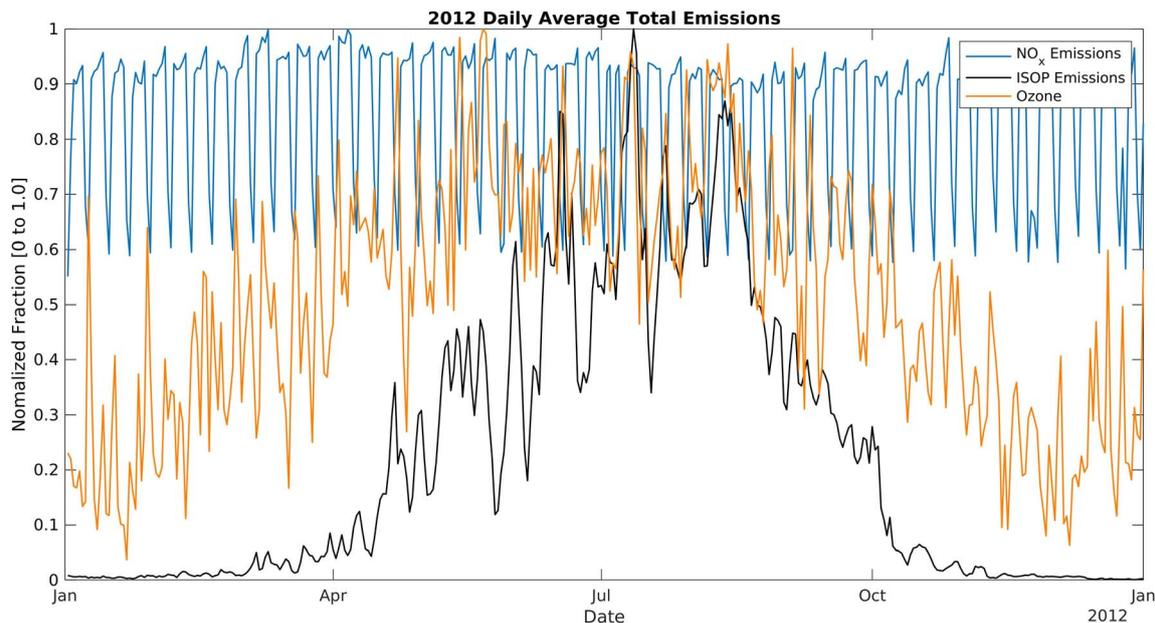
**Fig. 14** Daily average  $\text{NO}_x$  and isoprene (ISOP) emissions over the model domain normalized by the maximum value in the domain. The periodic oscillation of  $\text{NO}_x$  emissions (blue line) is due to weekday/weekend behavior. The black line is the biogenic isoprene emissions in the entire domain.  $\text{NO}_x$  and ISOP emissions were extracted from gridded SCAQMD emissions. Twenty-four-hour ozone averages were sampled from the Fontana air monitoring station.
