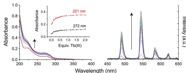
Fig. 1 Changes in (left) UV-Vis absorption and (right) phosphorescence spectra of an aqueous solution of **3Gal** on addition of Tb(CF<sub>3</sub>SO<sub>3</sub>)<sub>3</sub>. Inset: Binding isotherms.
