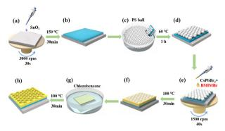
Fig. 1 Schematic diagram of the fabrication process for the CsPbBr<sub>3</sub> perovskite nanonet.
