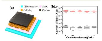
Fig. 3 (a) Schematic structure of the CsPbBr<sub>3</sub> nanonet PD. (b) Light and dark current statistics of the CsPbBr3 nanonet PDs with various concentrations of BMIMBr ionic liquid
