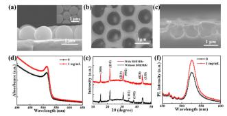
Fig. 2 (a) Cross-sectional SEM image of single-layer PS spheres; the inset shows the top view SEM image of single-layer PS spheres. Top (b) and cross-sectional (c) SEM image of the CsPbBr<sub>3</sub> perovskite nanonet film with BMIMBr ionic liquid. (d) Absorption spectra of the CsPbBr<sub>3</sub> perovskite nanonet films. (e) XRD patterns of the CsPbBr<sub>3</sub> perovskite nanonet films. (f) Steady-state PL spectra of the CsPbBr<sub>3</sub> perovskite nanonet films.
