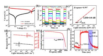
Fig. 4 The performance of the CsPbBr<sub>3</sub> nanonet PD with the optimal BMIMBr ionic liquid concentration (1 mg mL $^{-1}$ ): (a) I-V curves; (b) I-tcurves at different light intensities; (c) LDR; (d) R and D\*; (e)  $f_{-3dB}$ bandwidth; (f) response speed.
