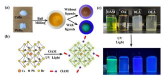
Fig. 1 (a) Photographs of the ball-milling processed Cs-Pb-Br perovskite emitter used in this study. (b) The schematic illustration of the lightemitting mechanisms for the OAM-functionalized perovskite emitters. (c) Photographs of the ambient light illuminated (upper c) and UV light illuminated (bottom c) different surfactant functionalized Cs-Pb-Br emitters dispersed in toluene.
