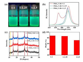
Fig. 3 (a) Photographs of the prepared Cs-Pb-Br NCs dispersed in toluene under UV light illumination. Different Cs/Pb material ratios were considered for comparison. (b) Steady-state PL spectrum, (c) XRD characterization, and (d) PLQY value of the Cs/Pb ratio dependent NCs.
