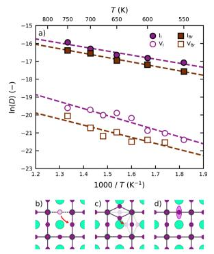
Fig. 3 (a) Temperature evolution of self-diffusion coefficients of halide vacancies (V<sub>X</sub>; white symbols) and halide interstitials (I<sub>X</sub>; coloured symbols) in CsPbX3. The defect migration pathways of (b)  $V_1$  and (c)  $I_1$  defects in CsPbI<sub>3</sub>, with both the initial and final structures. (d) The typical motion of halide species in the perovskite lattice.
