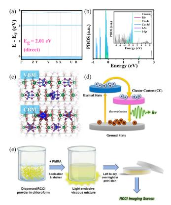
Fig. 2 (a) Electronic band gap structure. (b) PDOS of RCCI; the inset shows a PDOS with a larger range. (c) Plots of wavefunction  $|\Psi|^2$  of the CBM and VBM. (d) Schematic diagram of the photophysical processes. (e) Schematic illustration of the preparation procedure of RCCI@PMMA imaging screens.
