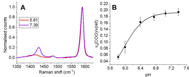
**Fig. 2** (A) SERS-MS spectrum at pH 5.81 and 7.06 after 14 days of simulated cell culture conditions in cell-free ECM. (B) pH calibration curve of SERS-MS in cell-free ECM after 14 days of simulated cell culture conditions.
