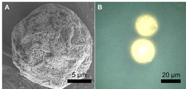
**Fig. 1** (A) Scanning electron microscope (SEM) image of dried SERS-MS. (B) Reflected brightfield microscope image of two SERS-MS in an aqueous solution.
