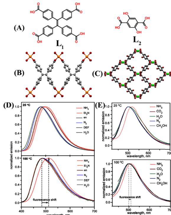
Fig. 1 (A) Molecular structure of ligands **L**<sub>1</sub> and **L**<sub>2</sub>. X-ray crystal structure of (B) LMOF **1** and (C) LMOF **2** (colour code: Zn orange, Mg green, O red, and C gray). Hydrogen atoms are not included for clarity. The relative changes in emission spectra of (D) **1** and (E) **2** when exposed to different analytes at 25 °C (top) and 100 °C (bottom). Reprinted with permission from ref. 47. Copyright 2013 American Chemical Society.
