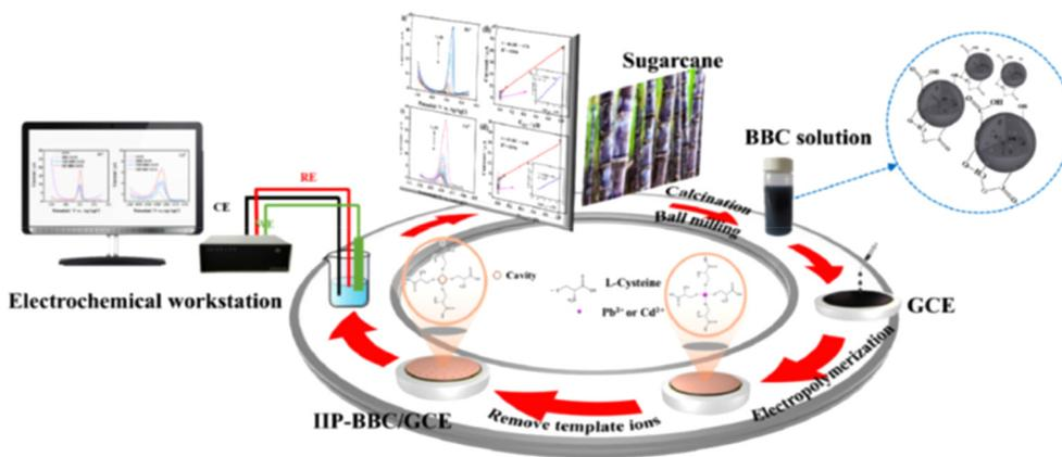
**Fig. 3** Schematic diagram for the preparation of the ion imprinted BBC electrode (IIP-BBC/GCE) and application for the detection of heavy metal ions<sup>219</sup> (this figure was published in D. Mao, J. Hu, P. Duan, C. Qin, Y. Piao, *Ultrasensitive and highly reusable electrochemical sensor with ion imprinted nanobiochar*, *Sens. Actuators, B*, **371**, 132490, Copyright Elsevier (2022)).
