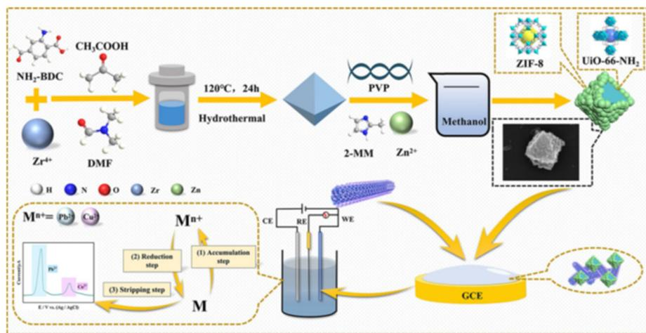
Fig. 5 The synthesis route of NU66@Z8 and the construction of the working electrode<sup>150</sup> (this figure was published in R. Tan, P. Jiang, C. Pan, J. Pan, N. Gao, Z. Cai, F. Wu, G. Chang, A. Xie, Y. He, Core-shell architected NH<sub>2</sub>-UiO-66@ZIF-8/multi-walled carbon nanotubes nanocomposite-based sensitive electrochemical sensor towards simultaneous determination of Pb<sup>2+</sup> and Cu<sup>2+</sup>, *Microchim. Acta*, **190**, 30, Copyright Springer (2023)).
