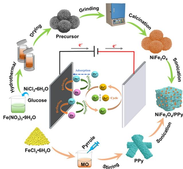
Fig. 2 Schematic illustration of the preparation process of the NiFe<sub>2</sub>O<sub>4</sub>/PPy nanocomposite.<sup>96</sup> Reprinted from Y. Wang, Z. Nie, X. Li, R. Wang, Y. Zhao, and H. Wang, PPy-functionalized NiFe<sub>2</sub>O<sub>4</sub> nanocomposites toward highly selective Pb<sup>2+</sup> electrochemical sensing, *ACS Sustainable Chem. Eng.*, 10(18), 6082–6093, Copyright (2022) American Chemical Society.
