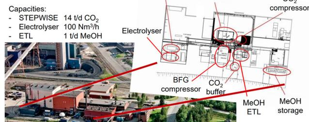
Fig. 21 Layout of the FReSMe project.<sup>89</sup>
