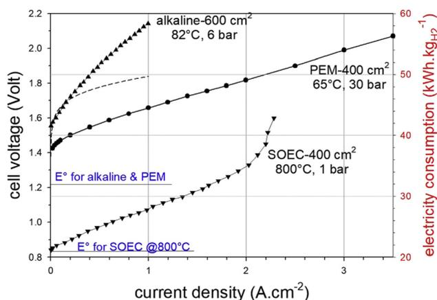
Fig. 4 Comparison of alkaline, PEM, and solid oxide electrolyzer cell (SOEC) technologies for electrolysis of water as a function of electricity consumption (current and voltage).<sup>51</sup> The indicative temperatures and pressures for each technology are a general representative of their operating conditions.
