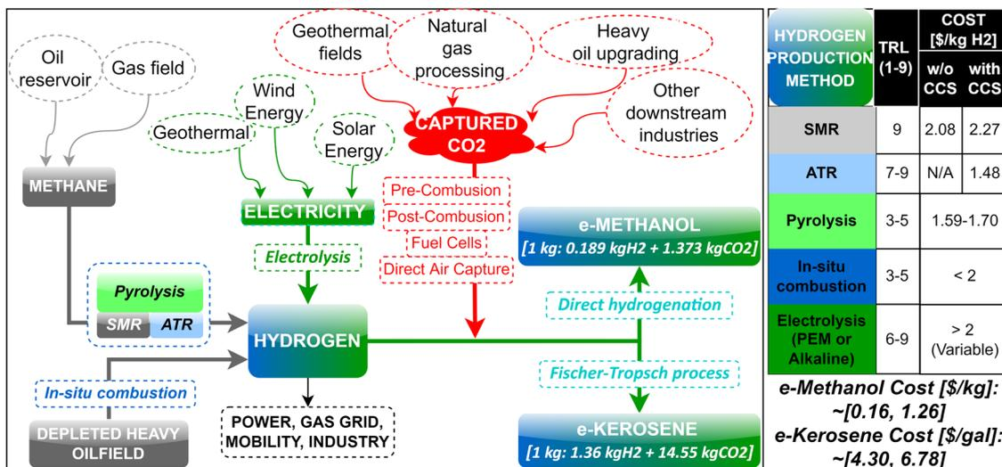
Fig. 3 A schematic illustrating the use of oil and gas resources to produce carbon-neutral liquid e-fuels. Hydrogen can be processed with captured CO<sub>2</sub> to produce carbon-neutral liquid e-fuels (e.g., e-methanol, e-kerosene) which (i) are compatible with existing engines, (ii) are easier to store, and (iii) can be transported using existing petroleum infrastructure.
