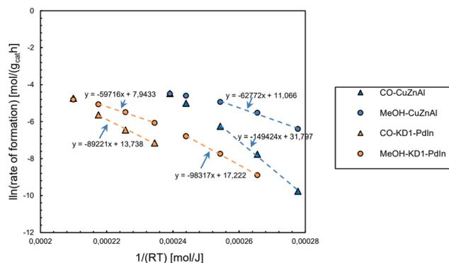
Fig. 12 Performance of selected catalysts in terms of the rate of production versus the input energy in the FRESMé project.<sup>89</sup>
