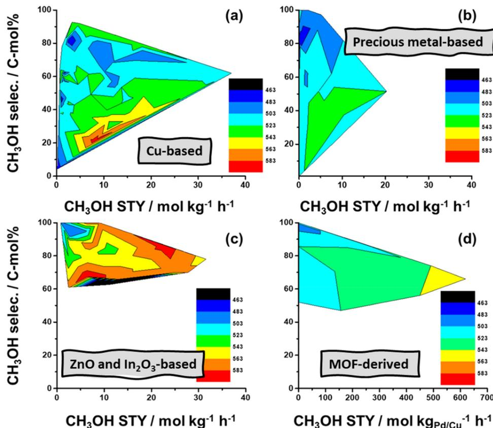
Fig. 11 Contour plots depicting catalytic performance in selectivity (conversion rate; in C-mol%) and space-time yield (STY; production rate; in  $\text{mol kg}^{-1} \text{h}^{-1}$ ) domain versus the reaction temperature (in K; color legend). The e-methanol production rate with MOF/ZIF-derived catalysts is normalized on active metals. Adapted from ref. 88.
