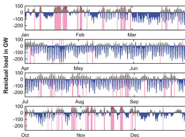
**Fig. 9** Simulated residual load profile (2050) with PtG operation (blue; negative residual load), GtP operation (grey; positive residual loads) and peak residual load management (red) for scenario 1. Pink vertical streaks indicate presence of peak residual load management.
