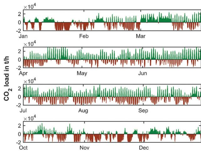
Fig. 10 Simulated CO<sub>2</sub> load profile (2050) for scenario 1.
