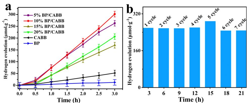
Fig. 5 (a) Yield of H<sub>2</sub> reduction by CABB, BP and the 10% BP/CABB composite after 3 h of photochemical reaction, error bar:  $\pm 0.03$ ; and (b) recycling test of the 10% BP/CABB composite.
