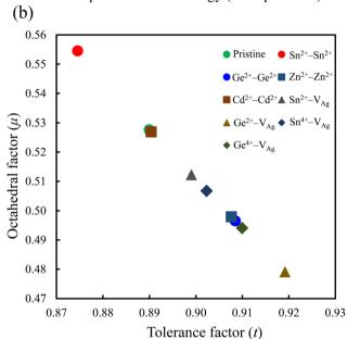
Fig. 2 (a) Dopant formation energy vs. decomposition energy, and (b) tolerance factor vs. octahedral factor for the perovskite structures. The filled and empty symbols in (a) represent the decomposition energy using the path in eqn (7) and (8), respectively.
