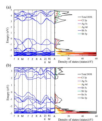
Fig. 3 Band structure (left) and density of states (right) of (a) the pristine perovskite and (b) the Sn<sup>2+</sup>-Sn<sup>2+</sup> doped perovskites.
