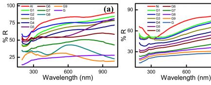
Fig. 4 Optical reflectance spectra of (a) G: Al and (b) G: Ni electrodes.
