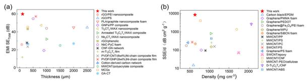
Fig. 4 Comparison of the EMI shielding performance. (a) EMI SE<sub>Total</sub> versus the thickness of  $Ti_3C_2T_x/MLPAN$  and other EMI shielding materials from the references. (b) Thickness-normalized specific SE (SSE/d) of  $Ti_{\tau}C_{2}T_{\nu}/MLPAN$  with a density of 639.0 mg cm<sup>-3</sup> and other EMI shielding materials from the references
