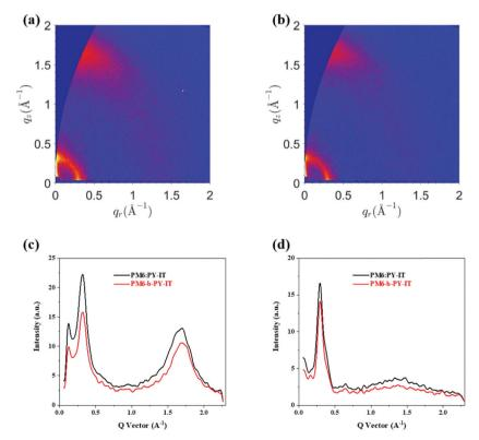
Fig. 2 The 2D-GIWAXS patterns of (a) PM6:PY-IT and (b) PM6-b-PY-IT. Intensity profiles based on the (c) OOP and (d) IP directional diffraction signals.
