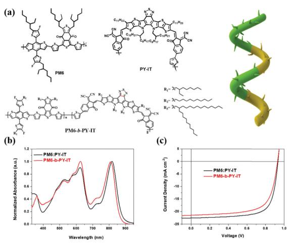
Fig. 1 (a) Chemical structures of the materials used in this work. (b) Normalized UV-vis absorbance spectra of the two systems. (c) The J-Vcharacteristics of the materials
