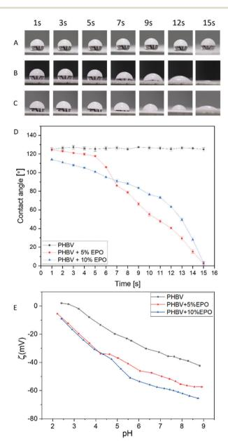
Fig. 5 The representative images of water drops on (A) PHBV fibers and (B) blend PHBV fibers with 5% EPO and (C) 10% EPO. (D) The change in water contact angle on the PHBV fibers and blends of PHBV fibers with 5% and 10% EPO within 15 seconds. (E) Zeta potential (ζ) results showing titration curves for the PHBV fibers and blends of PHBV fibers with 5% and 10% EPO measured in KCl solution.
