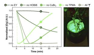
Fig. 5 Oxygen concentration measurements. Reactions conditions:  $[HOBiB]/[EYH_2]/[CuBr_2]/[TPMA] = 1/0.01/0.2/0.6$ , [HOBiB] = 1.5 mM, in PBS with DMSO (10% v/v), irradiated for 30 min under green LEDs (520 nm, 9.0 mW cm<sup>-2</sup>) in an open vial with stirring at 500 rpm.
