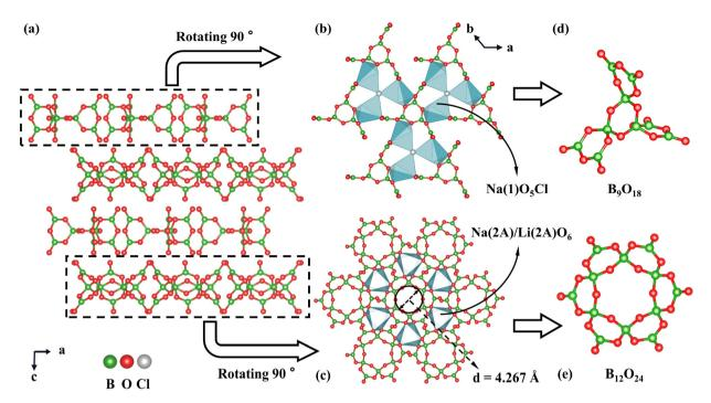
Fig. 3 The crystal structure of LNSBOC. (a) View of the layer-like structure along the b-axis; (b) the plane consists of fan-like B<sub>9</sub>O<sub>18</sub> groups; (c) the plane consists of petal-like  $B_{12}O_{24}$  groups; (d) isolated  $B_9O_{18}$  cluster; (e) isolated  $B_{12}O_{24}$  cluster.
