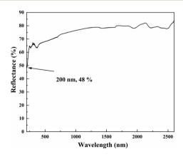
Fig. 6 The UV-vis-NIR optical spectrum of LNSBOC.
