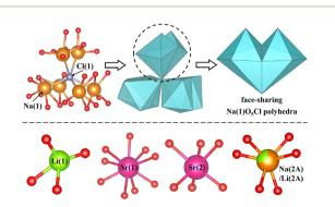
Fig. 2 Face-sharing Na(1)O<sub>5</sub>Cl polyhedra and the coordination environments of the Li, Na and Sr atoms in the title compound.
